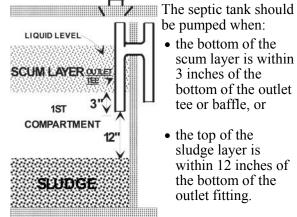
• the top of the sludge layer is within 12 inches of the bottom of the outlet fitting.
